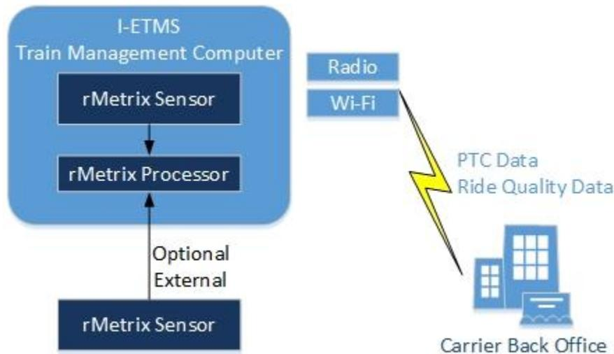
*Figure 3 – I-ETMS PTC System and rMetrix Ride Quality Integration*
