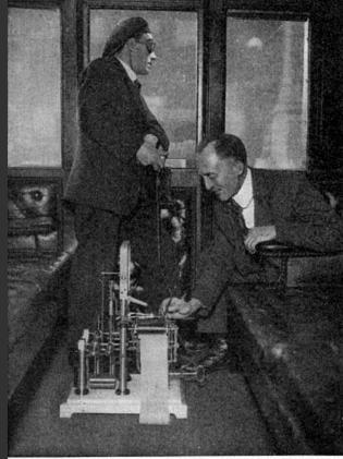
FIG. 55 .- Using the Hallade track recorder.
